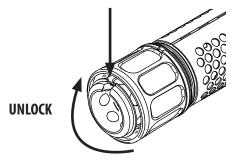
4 Pull the suppressor back onto the muzzle device so the alignment notch and the alignment pin achieve the 12 o'clock position.
